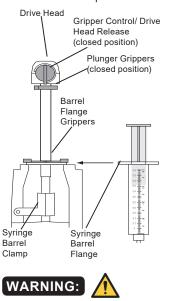
Before loading or unloading the syringe, always turn off fluid flow to the patient, using the tubing clamp or stopcock. Uncontrolled fluid flow can occur when the infusion set is not clamped or turned off, and can cause serious injury or death.
