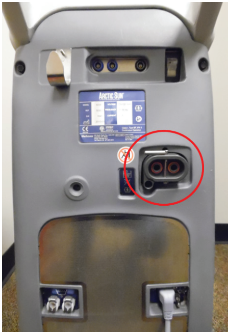
Figure 2.4. ARCTIC SUN® Temperature Management System Control Module with fluid delivery line removed
