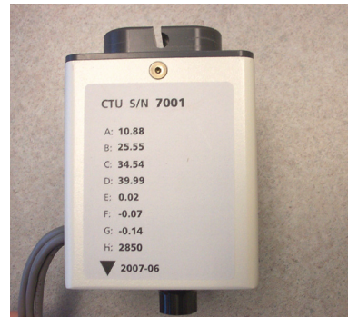
Figure 2.8. CTU calibration data
