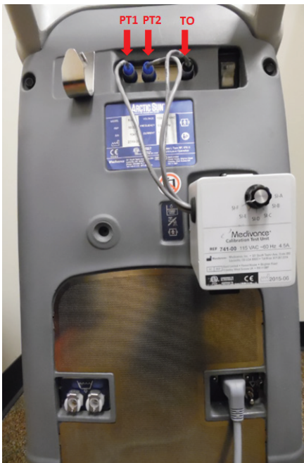
Figure 2.5. ARCTIC SUN® Temperature Management System Control Module with CTU attached
